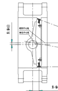
Triple Eccentric Structure Diagram. Its main characteristic is turning with 0 friction, the torque generates resilient seal.
